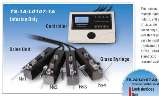
The pumps combine precison, compact size, multiple functions with ease of operation. It can hold µL unit standard glass syringe. The features of accurate distance control and broad linear speed range (7.9µm/min-79.4mm/min) can meet versatile requirements. The drive unit is separate, easy to installation and combination. Its vertical (horizontal) installation structure makes this pump easily used in micromanipulator, stereotaxic instrument for various biologic research applications.
